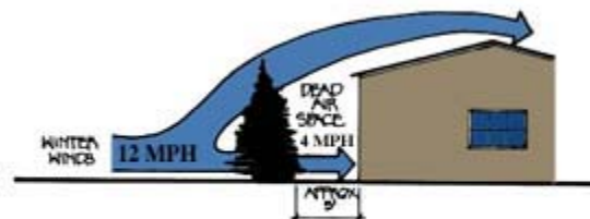
Figure 8. Evergreens adjacent to the north and west sides of a house reduce wind speed and create dead air space for insulation.
